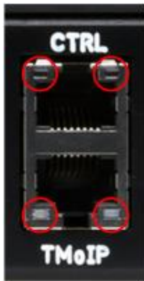
Figure 8: Back Panel RJ-45 CTRL and TMoIP Ports, LEDs
