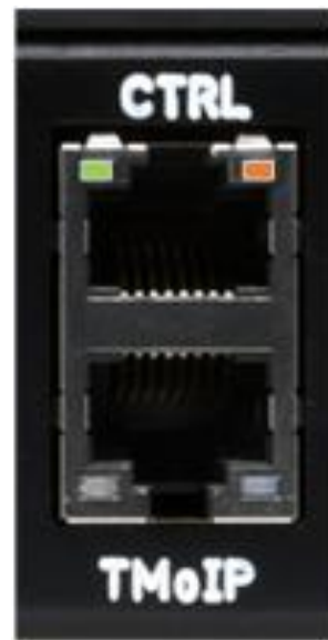
Figure 9: CTRL and TMoIP Ports, Example Green and Orange LEDs
