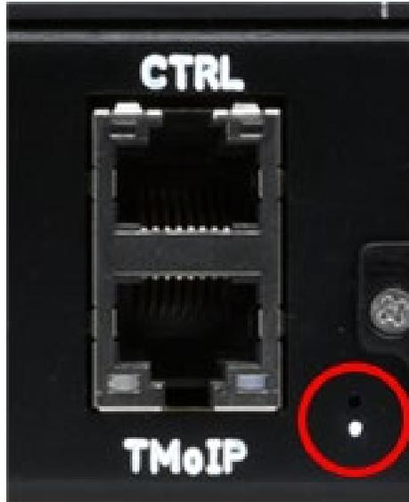
Figure 10: Back Panel Reset Button Access
