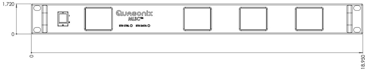
**Figure 2: Mechanical Drawing – 1U Front View**
