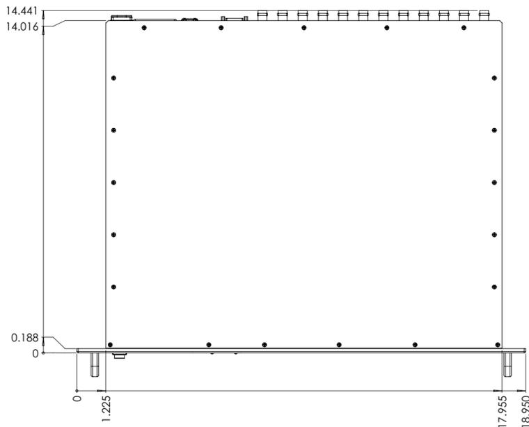
**Figure 4: Mechanical Drawing – 1U Top View**
