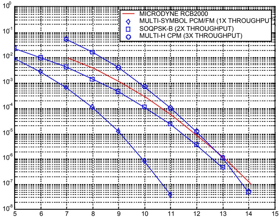
Figure 9. Bit Error Rate Performance of the MMD22.
