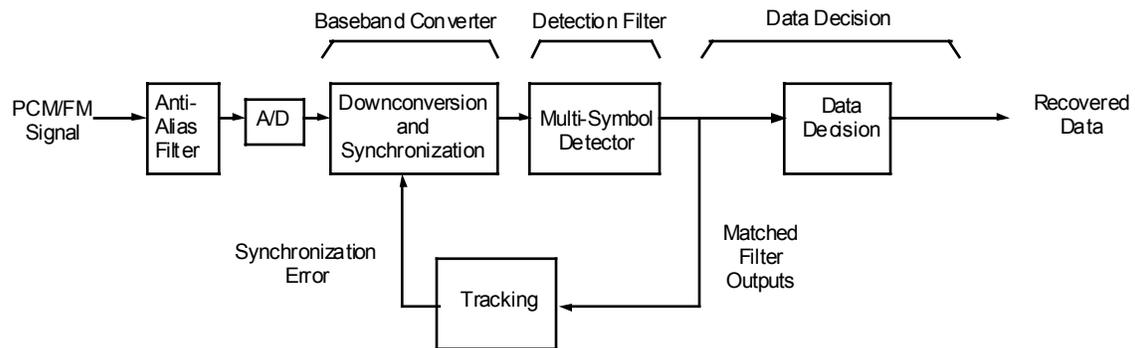
**Figure 6. PCM/FM (Tier 0) Configuration**
