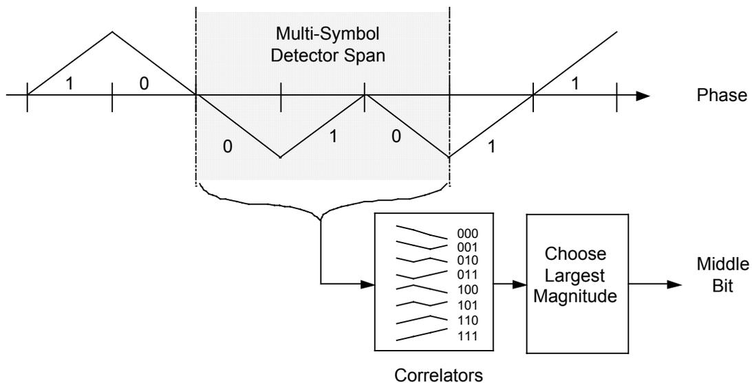
**Figure 7. Multi-symbol Detection Approach for PCM/FM.**
