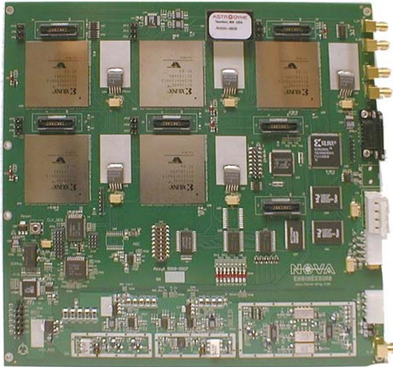
Figure 8. Signal Processing Board in the MMD2.
