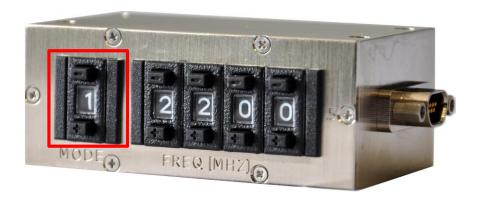
Figure 3: Front Close-up of Switch Box, Mode Digit Highlighted
