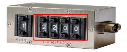
Figure 2: Front Close-up of Switch Box, Frequency Digits Highlighted
