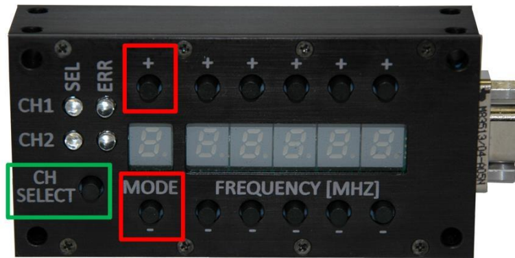
Figure 14: Increase LED Display Brightness Key Press Example
