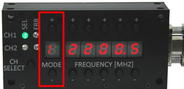
Figure 5: 2 nd Generation Switch Box Mode Selection
