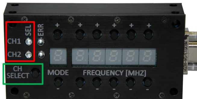
Figure 2: 2 nd Generation Switch Box Channel Selection
