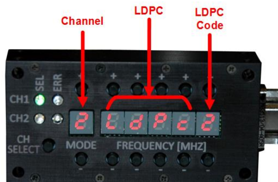
Figure 8: Labeled LDPC Display Example, Channel 2, LDPC Code 2
