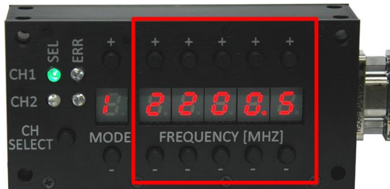
Figure 6: 2 nd Generation Switch Box Frequency Selection
