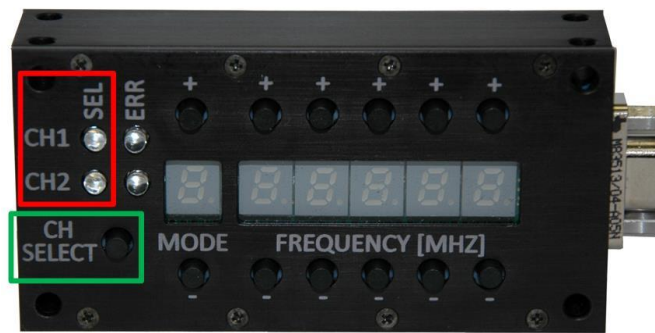
Figure 2: 2 nd Generation Switch Box Channel Selection
