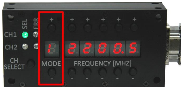
Figure 5: 2 nd Generation Switch Box Mode Selection
