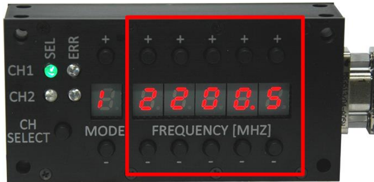
Figure 6: 2 nd Generation Switch Box Frequency Selection
