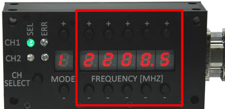
Figure 6: 2 nd Generation Switch Box Frequency Selection
