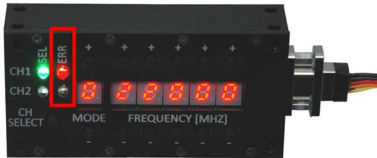
Figure 10: 2 nd Generation Switch Box Error LEDs, One Glowing Red
