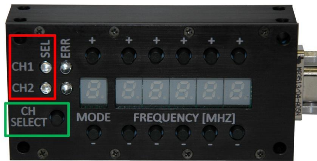
Figure 2: 2 nd Generation Switch Box Channel Selection
