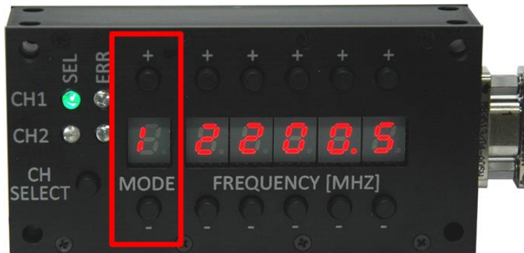
Figure 5: 2 nd Generation Switch Box Mode Selection
