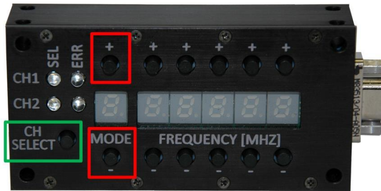
Figure 14: Increase LED Display Brightness Key Press Example
