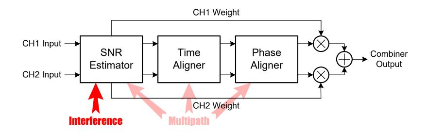
Inaccurate SNR estimation: overwhelm estimator with strong undesired signal
