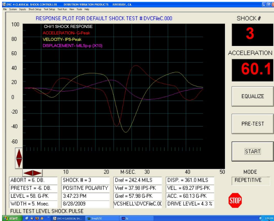
Figure 37: Shock Pulse, Z-axis Positive
