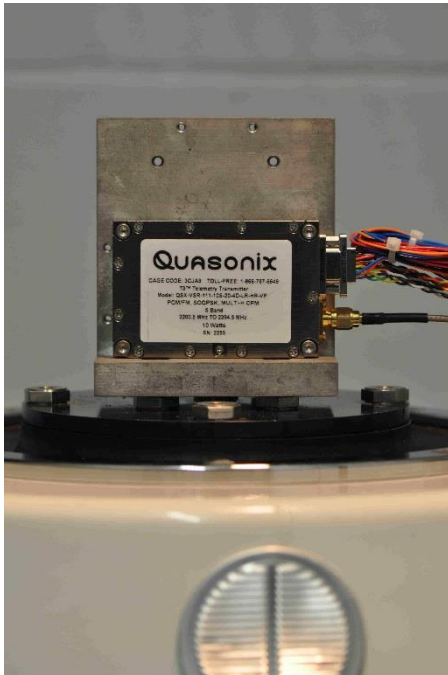
Figure 31: TIMTER™ Mounted for X-axis Testing
