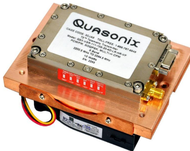
Figure 5: Fan-cooled Heat Sink with 6 cubic inch TIMTER™
