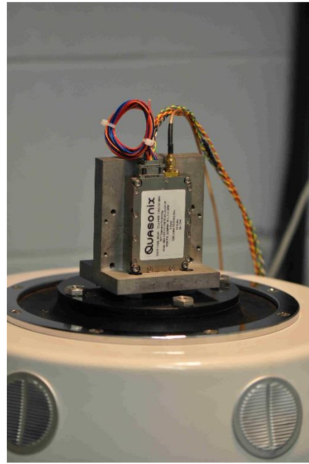
Figure 32: TIMTER™ Mounted for Y-axis Testing
