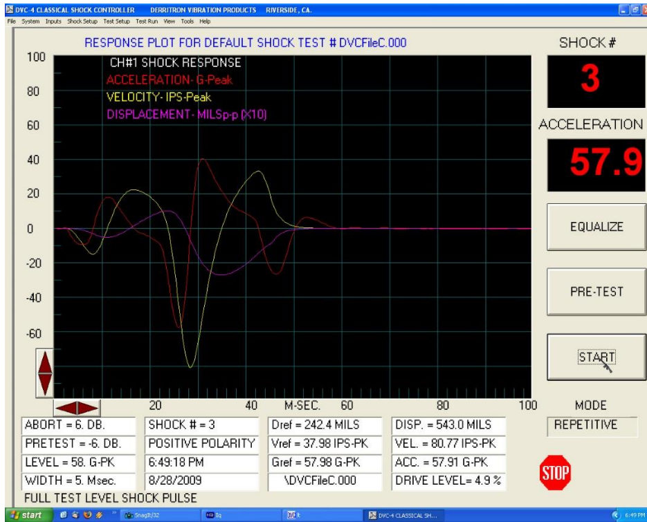
Figure 41: Shock Pulse, X-axis Positive
