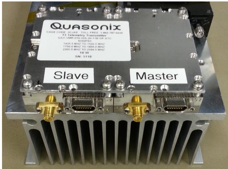
Figure 13: Legacy Dual Telemetry Transmitter Mounted Example
