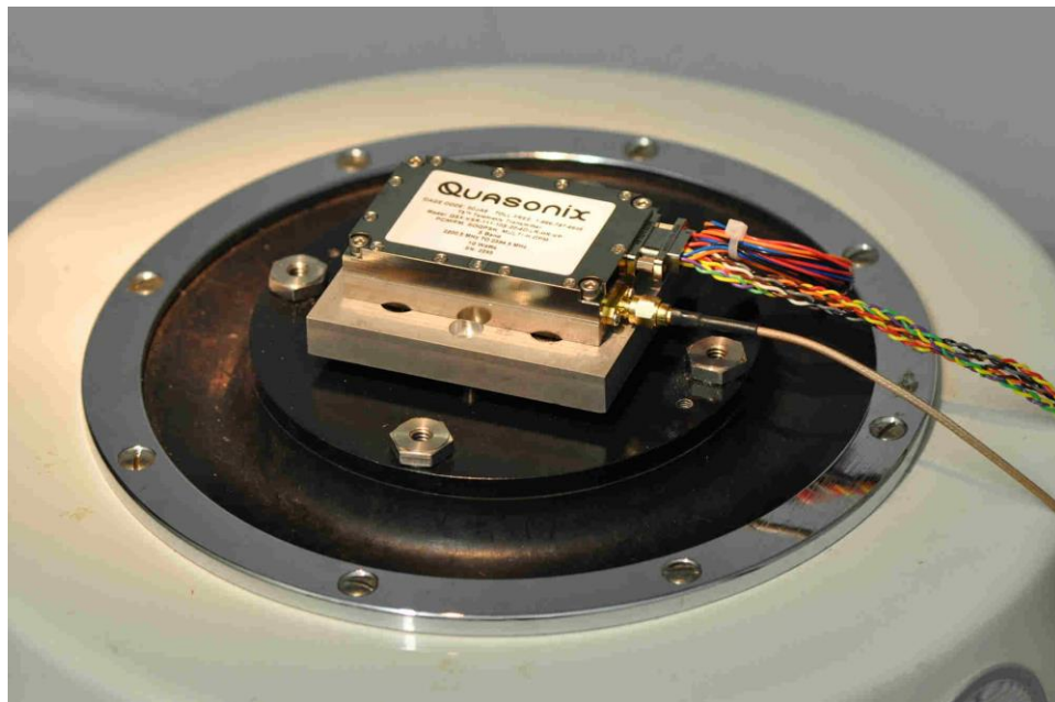
Figure 34: TIMTER™ Mounted for Z-axis Testing
