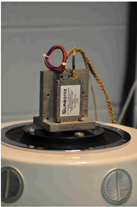
Figure 36: TIMTER™ Mounted for Y-axis Testing
