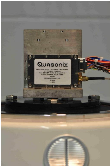
Figure 35: TIMTER™ Mounted for X-axis Testing
