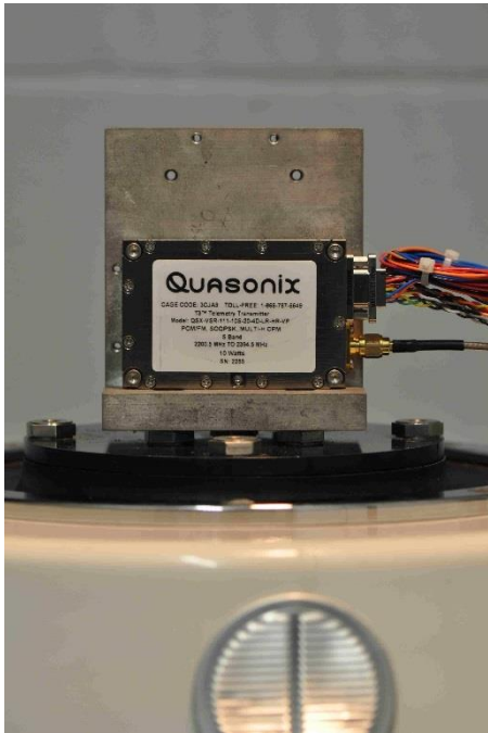
Figure 35: TIMTER™ Mounted for X-axis Testing
