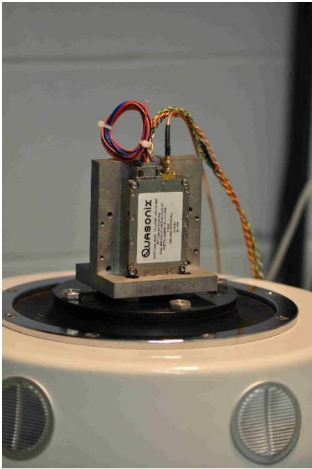
Figure 36: TIMTER™ Mounted for Y-axis Testing
