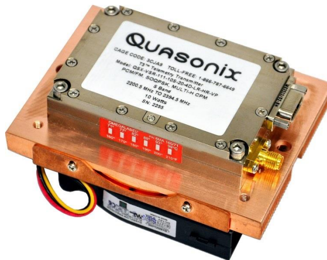
Figure 4: Bench Heat Sink shown with 6 cubic inch TIMTER™
