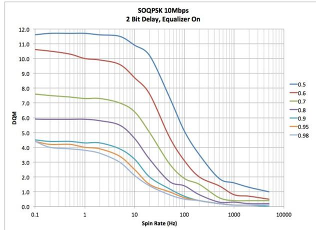
Figure 11 - Equalizer Break Frequency Test Results.
