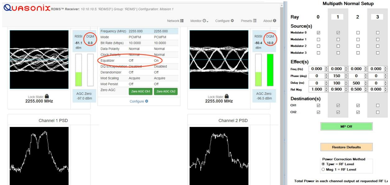
Figure 5 - Eye Pattern and Spectrum, Before and After Equalization.
