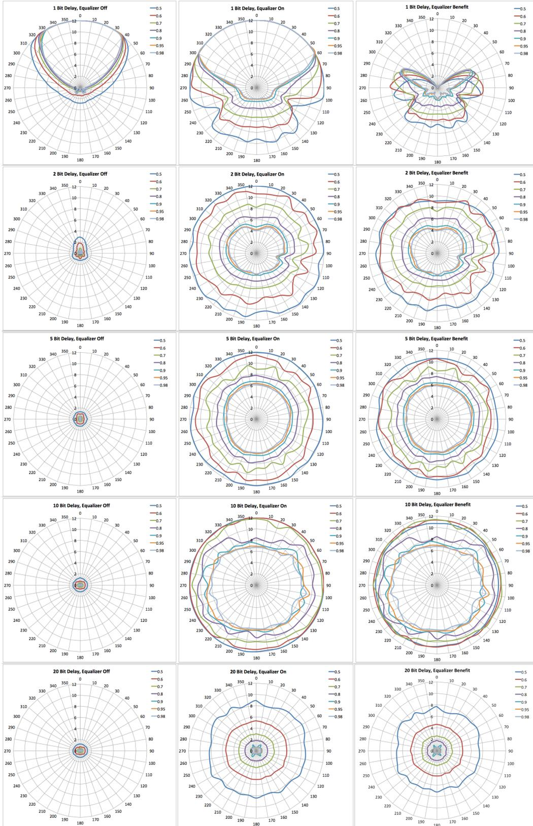
Figure 10 - Equalizer Benefit Plots, 10 Mbps SOQPSK, Delays of 1, 2, 5, 10, and 20 bits.
