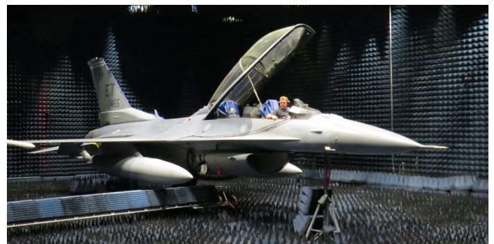
An F-16, used to test two-antenna interference and STC (chart at left), is mounted in the JPRIMES anechoic chamber at Eglin Air Force Base.
