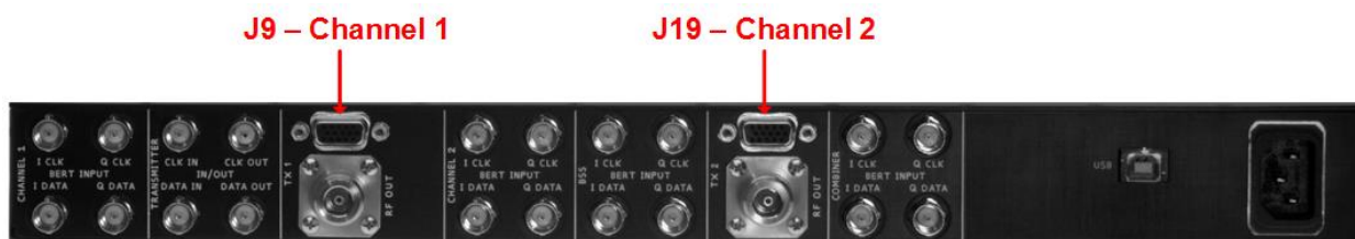
Figure 4: RA Back Panel, J9 and J19 Labeled
