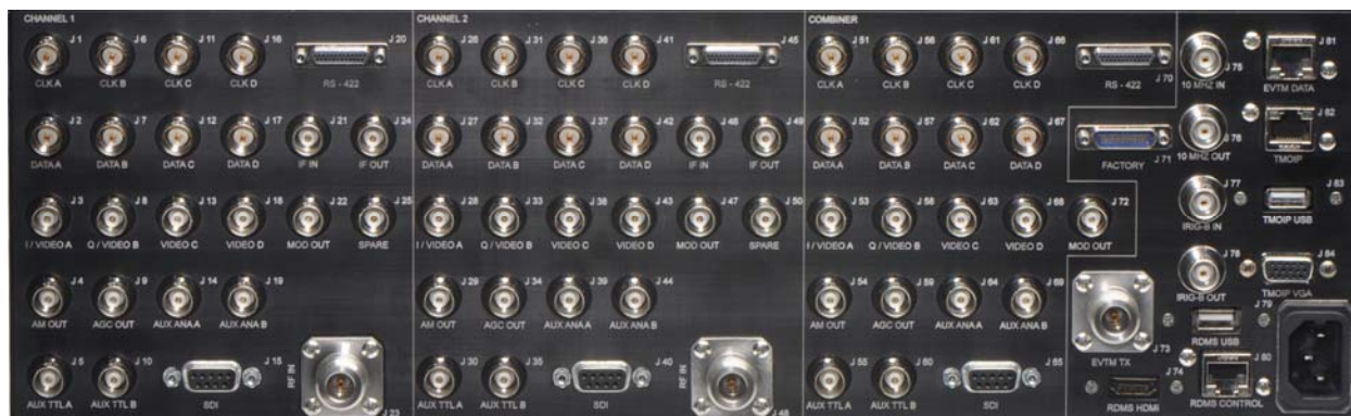
Figure 201: 3 rd Generation RDMS 3U Back Panel Connectors
