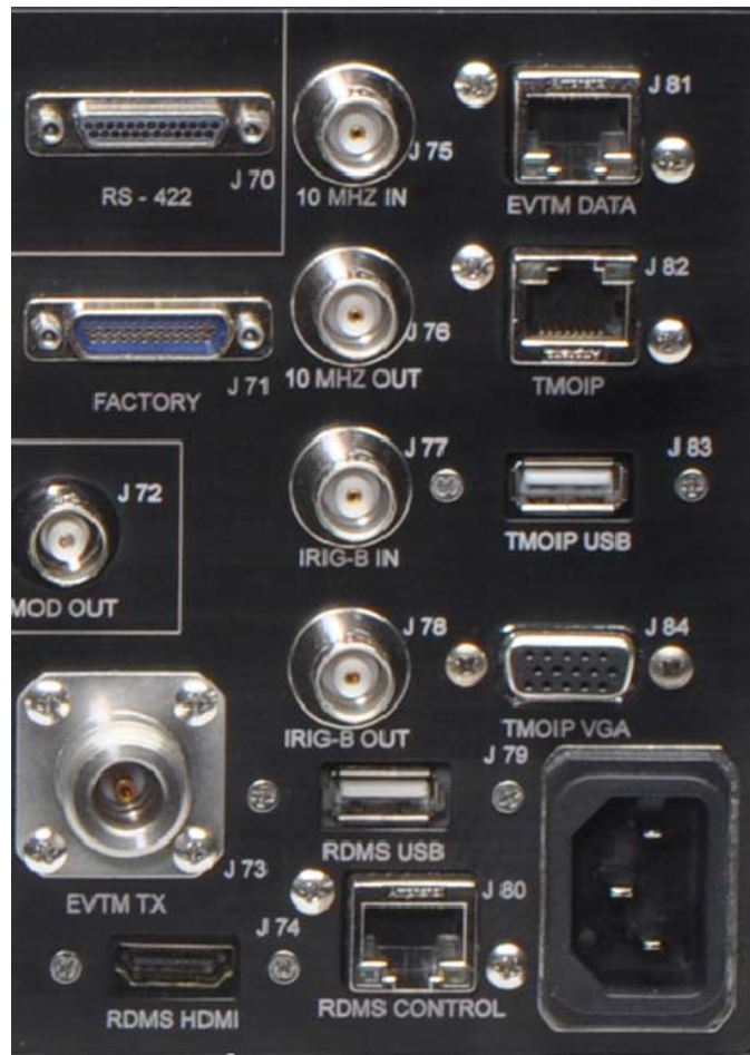
Figure 202: 3 rd Generation RDMS 3U Back Panel Connectors-Right Side
