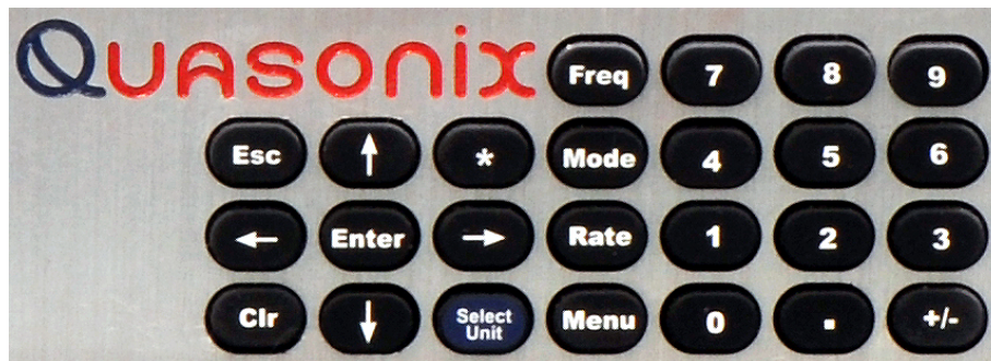
Figure 11: Front Panel Keypad
