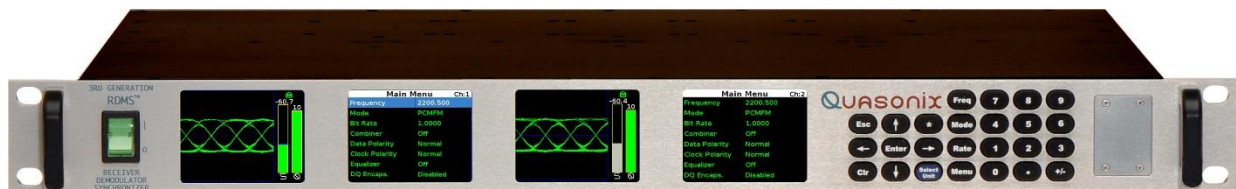
Figure 12: Front Panel Diagram for Dual-Channel Configuration
