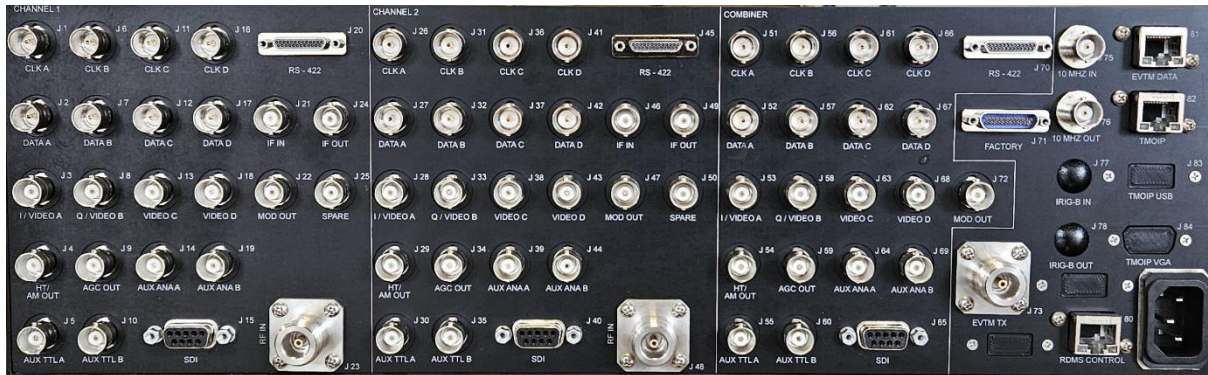
Figure 314: 3rd Generation RDMS 3U with IP2 Option, Back Panel Connectors
