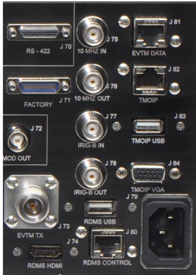
Figure 354: 3rd Generation RDMS 3U Back Panel Connectors-Right Side
