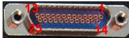
Figure 9: 1U Rear Panel Female MDM-25 D-Sub Connector for J31, Pins Labeled
