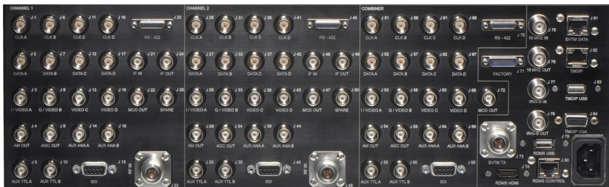
Figure 346: 3rd Generation RDMS 3U Back Panel Connectors
