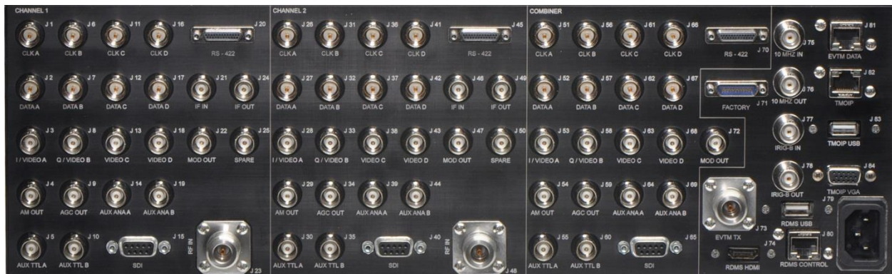
Figure 320: 3rd Generation RDMS 3U with IP Option, Back Panel Connectors
