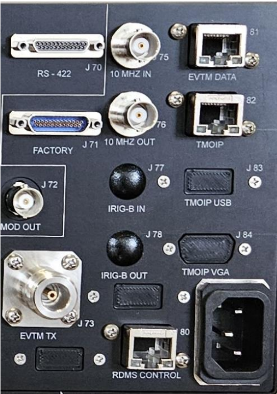
Figure 315: 3rd Generation RDMS 3U with IP2 Option, Back Panel Connectors-Right Side
