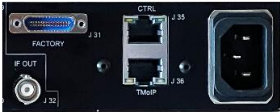
Figure 316: 3rd Generation RDMS 1U with IP2 Option, Back Panel Connectors-Right Side
