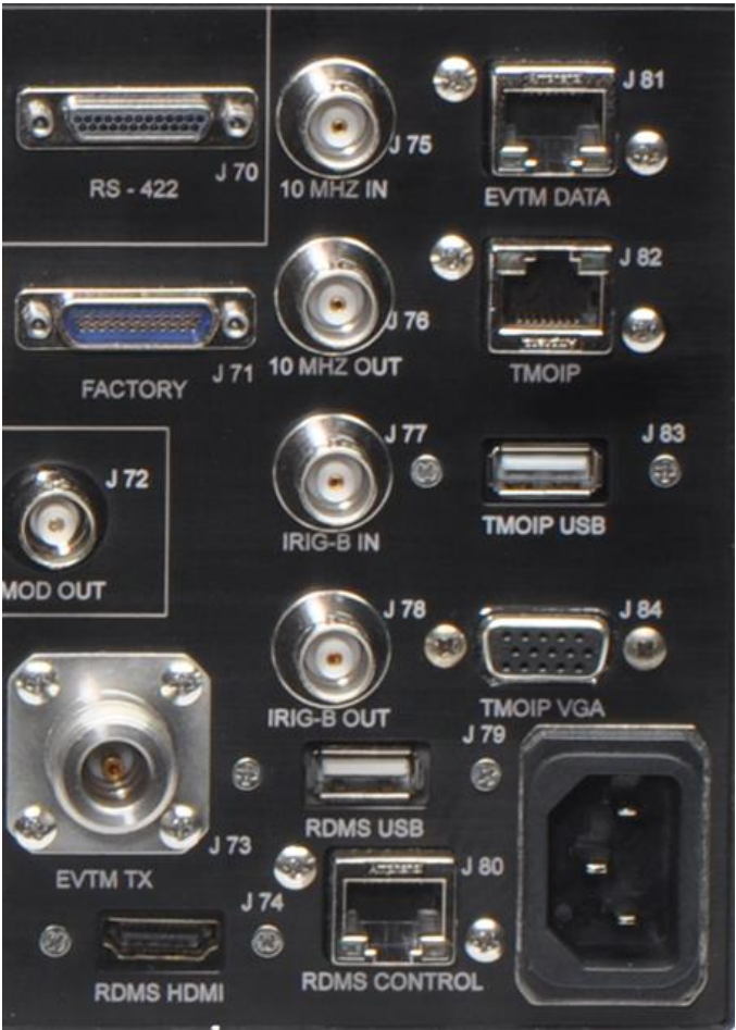
Figure 313: 3rd Generation RDMS 3U Back Panel Connectors-Right Side
