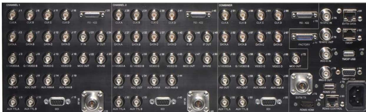
Figure 212: 3 rd Generation RDMS 3U Back Panel Connectors
