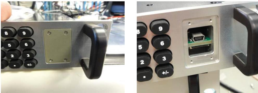
Figure 1: Front Panel, USB/Micro SD Port Access
