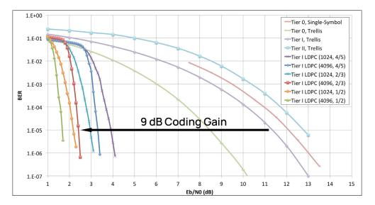
**Improves Link Margin by 8.8 to 9.4 dB at BER = 1e-5** – Link margin improvement is equivalent to nearly tripling the operating distance on your telemetry link.
