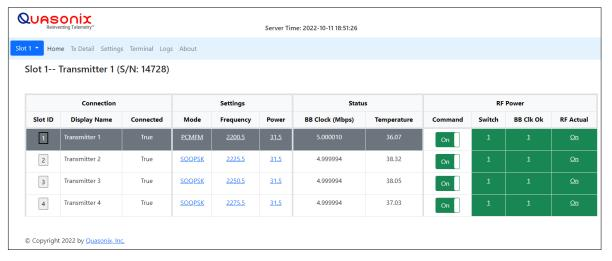
Browser-based GUI facilitates monitoring status and controlling up to four transmitters at one time.
