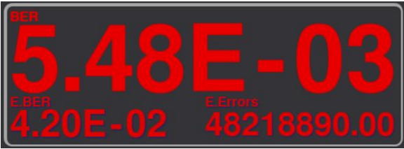
Figure 58: Red: BERT Pattern Sync Failure; DQE Mode On with No Frame Sync
