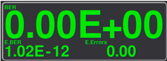
Figure 57: Green: BERT Pattern Sync/DQE Frame Sync Achieved
