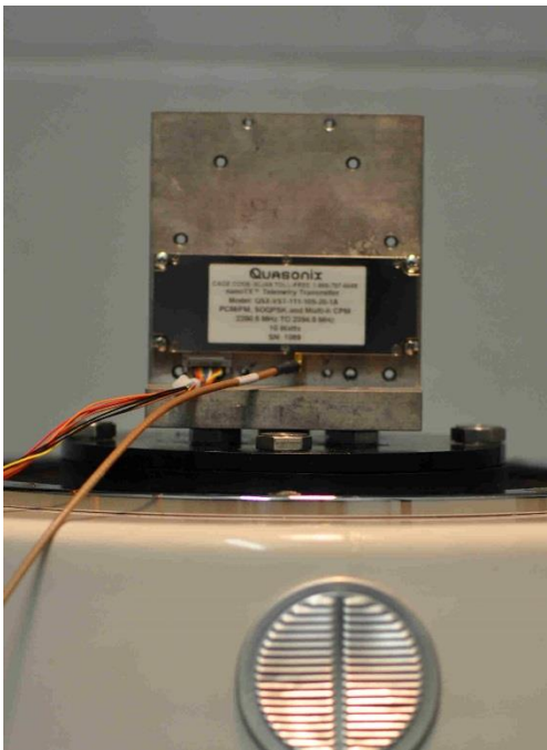
Figure 29: nanoTX™ Mounted for X-axis Testing
