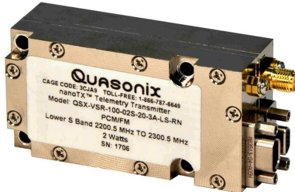
Figure 6: 3.6 in³ GMLRS Transmitter
