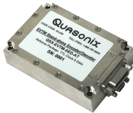
Figure 1: EVTM Stand-alone Encoder/Decoder for Airborne Applications
