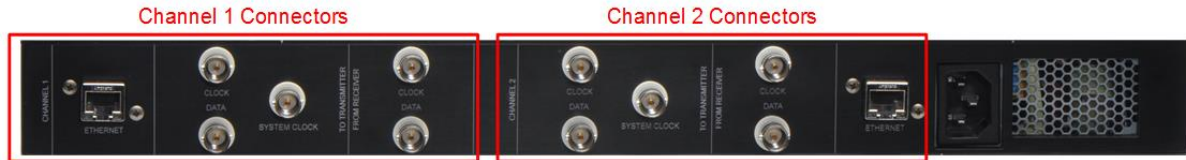
Figure 8: Rack Mount EVTM Encoder/Decoder with Channels Labeled
