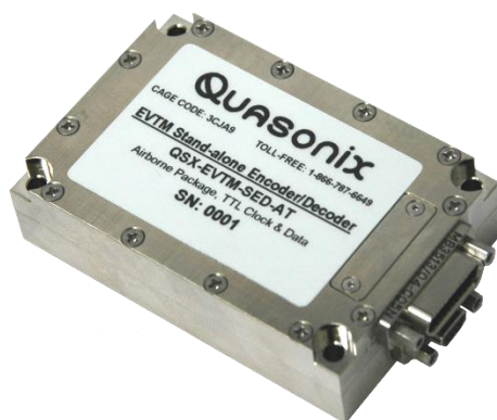
Figure 5: 4.2 in3 Airborne Encoder/Decoder
