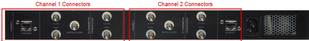
Figure 8: Rack Mount EVTM Encoder/Decoder with Channels Labeled
