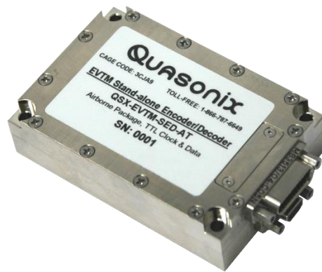
Figure 1: EVTM Stand-alone Encoder/Decoder for Airborne Applications
