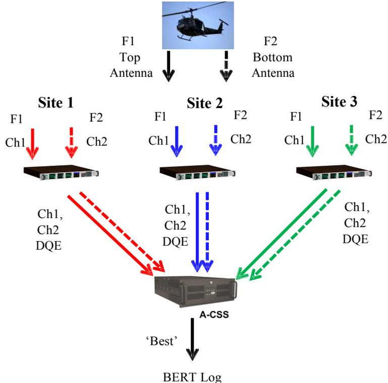
**Figure 6: High Level BSS Test Setup**
