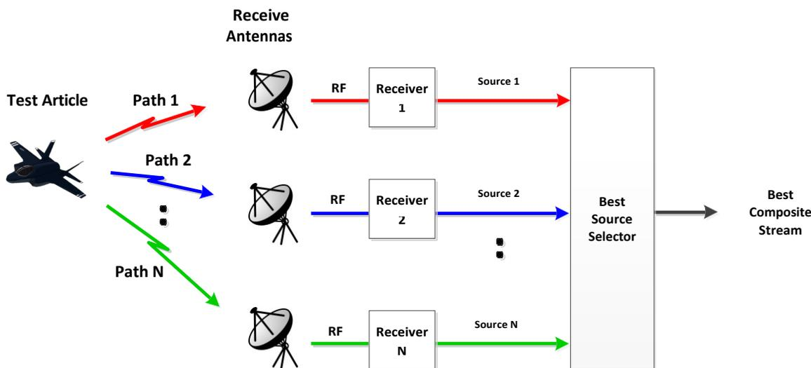
Figure 1: Best Source Selector System Diagram
