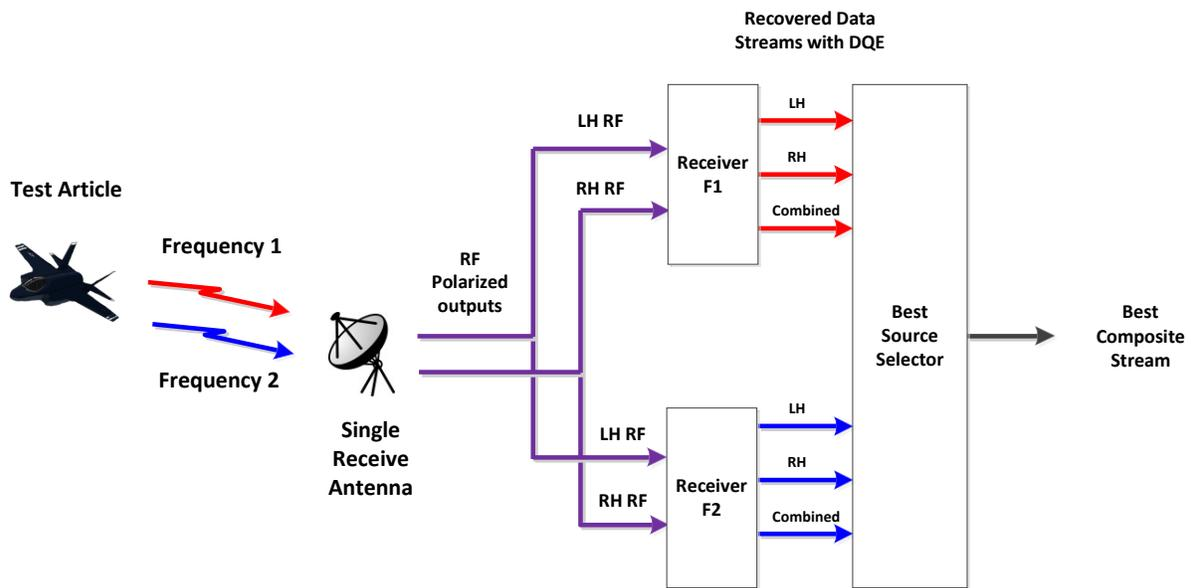
**Figure 9: Single Site BSS example using both Frequency and Polarization Diversity**
