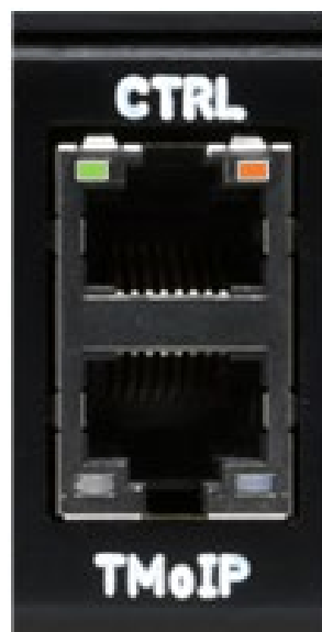
Figure 8: CTRL and TMoIP Ports, Example Green and Orange LEDs
