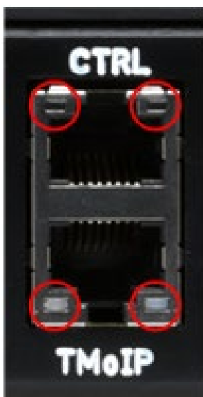
Figure 7: Back Panel RJ-45 CTRL and TMoIP Ports, LEDs
