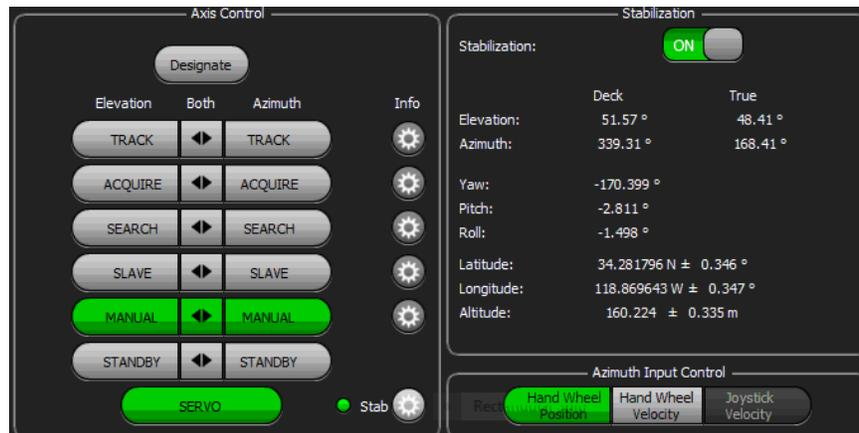
Figure 128: Stabilization Window with Stability Enabled (On), All Parameters Present and Reliable
