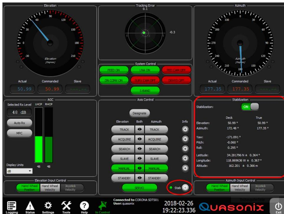
Figure 123: ACU Front Panel with Stability Selected
