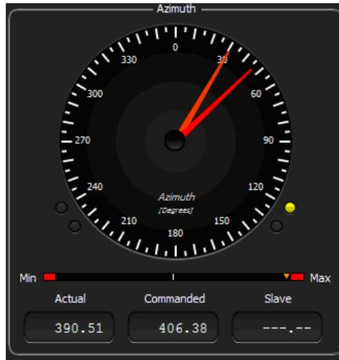
Figure 67: Azimuth Axis Position Dial with Cable Wrap Meter Enabled
