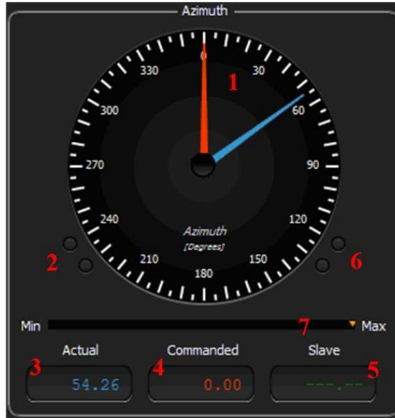
Figure 6: Azimuth Axis Analog/Digital Position Feedback Display
