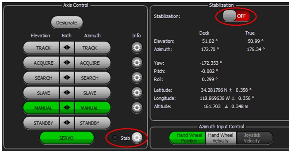
Figure 124: Stab Button and Stabilization Window On/Off Selection
