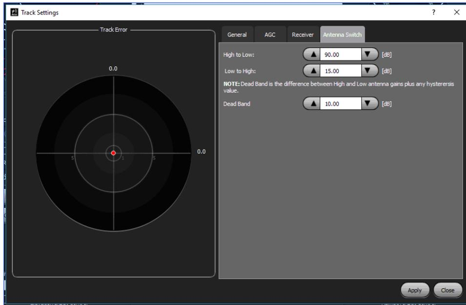
Figure 83: Track Settings Dialog Box, Antenna Switch Tab
