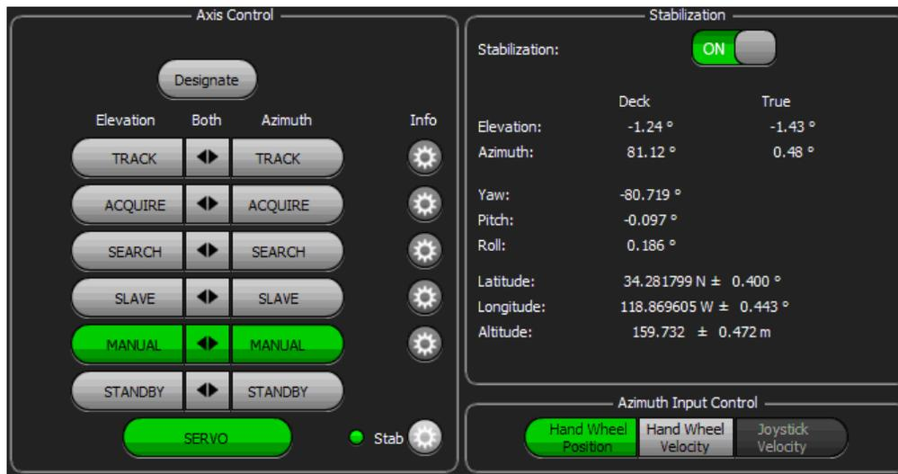
Figure 20: Axis Control and Stabilization Windows, Stabilization Option Enabled and Switched On
