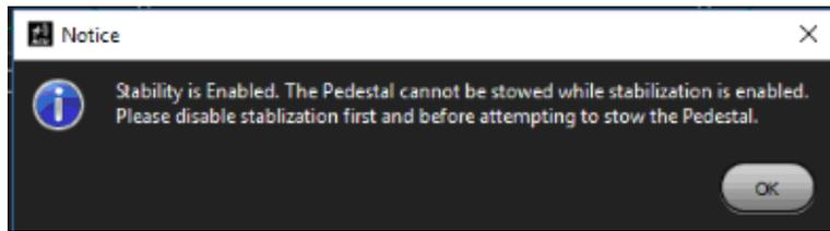
**Figure 15: Stow Warning Message When Stability Enabled**
