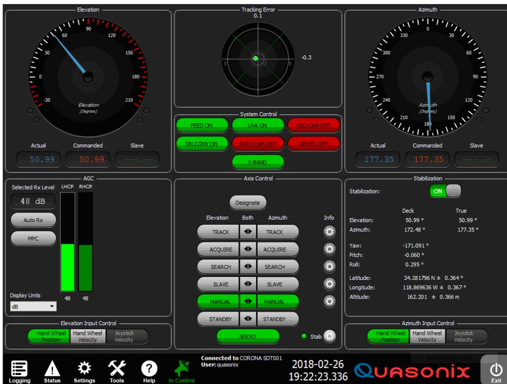
Figure 9: Quasonix ACU Front Panel Display, Stability Enabled
