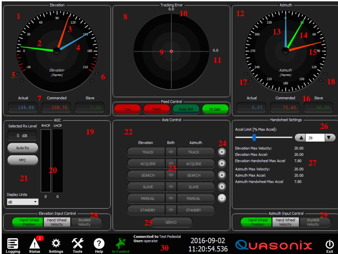
Figure 111: ACU Front Panel GUI with Parts Numbered
