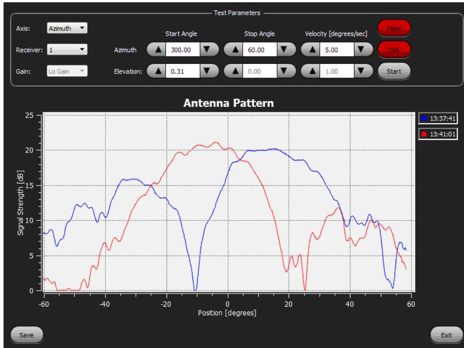
Figure 94: Test Parameters/Antenna Pattern Test Dialog Box
