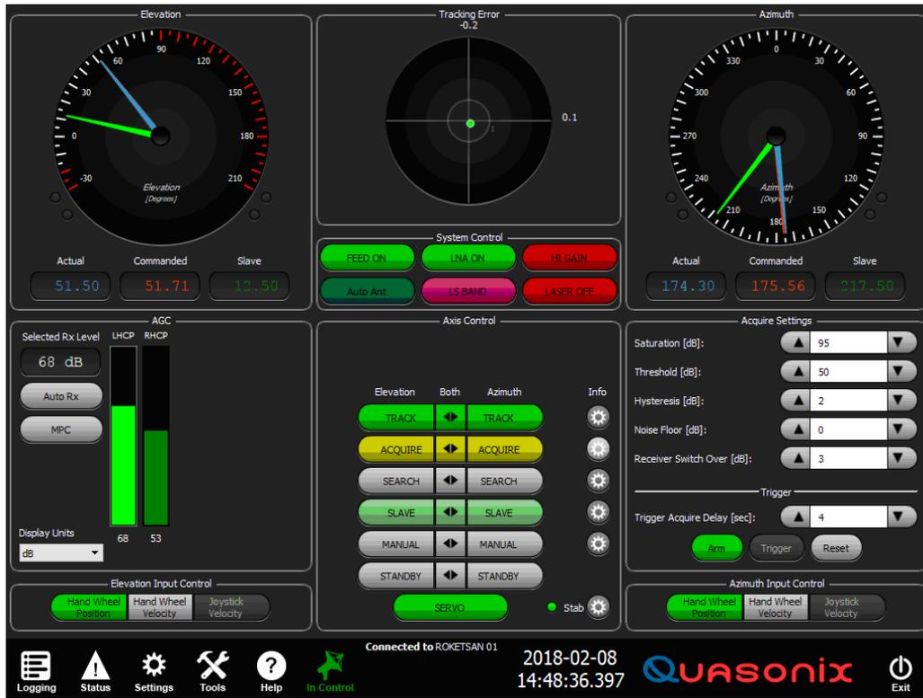
Figure 132: ACU Front Panel, External Trigger Pulse Received
