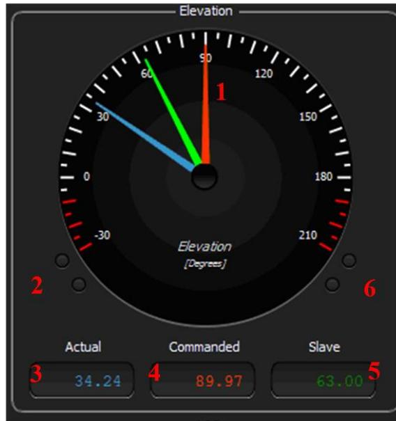
Figure 5: Elevation Axis Analog/Digital Position Feedback Display
