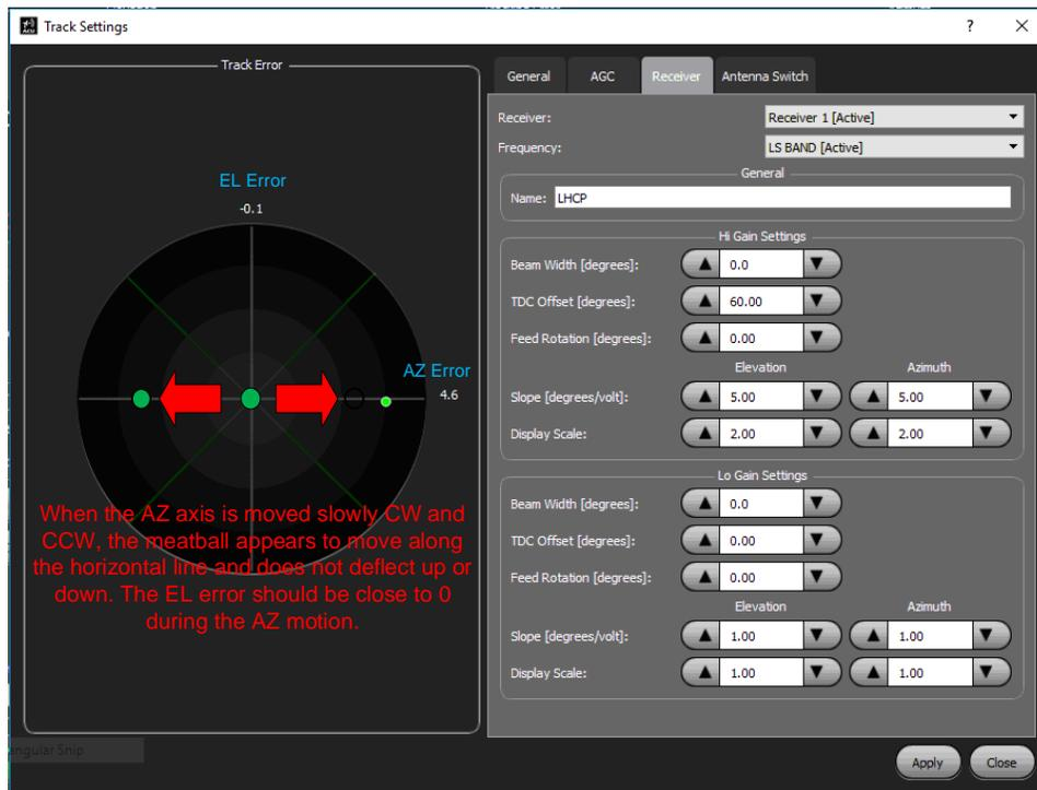
Figure 112: Track Settings Condition 1-Adjusting TDC Offsets
