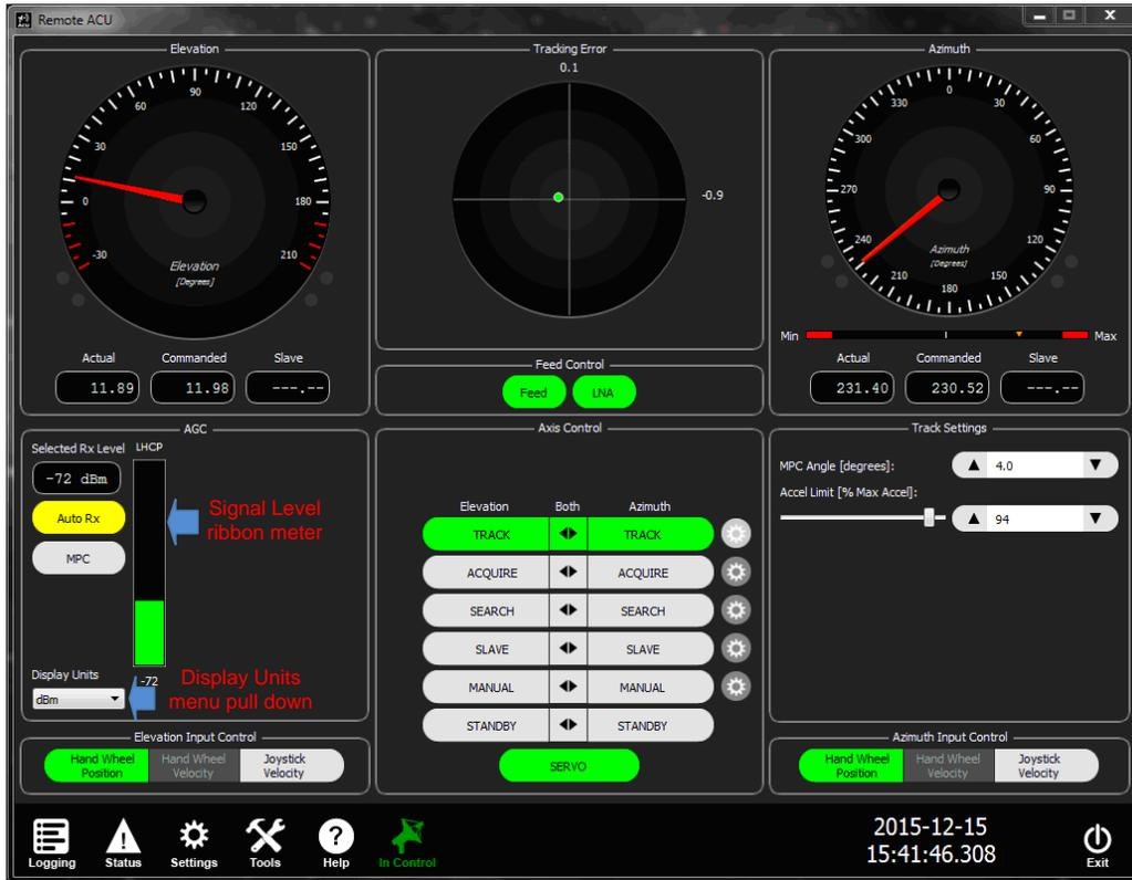
Figure 119: ACU Front Panel, AGC Window Labeled
