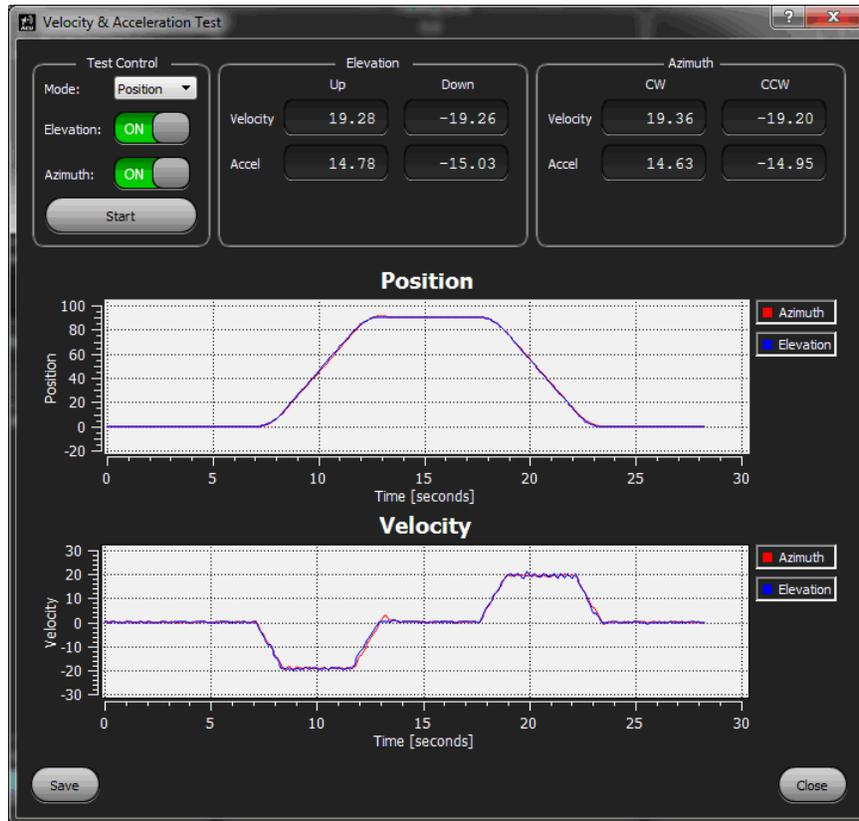
Figure 93: Velocity & Acceleration Test Dialog Box
